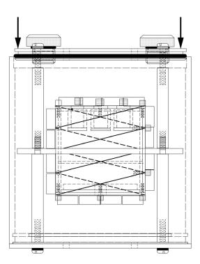
To install the test cube and support disk, the two pieces of the support disk need to be oriented so the wide flanges correspond to the notches in the test cube. Then attache the retaining disks. The cube and disk assembly should then be lowered onto the support posts in the phantom.
