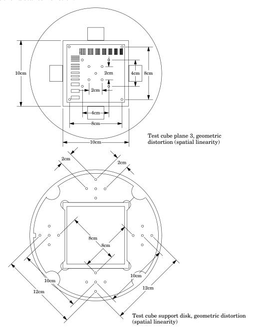
For larger field measurements of geometric distortion use the test cube support disk which is positioned 1.25cm above this test plane.
