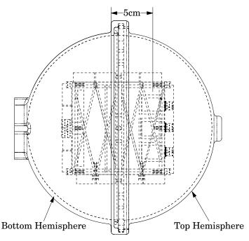
With the Magphan® cylinder, align the light with the top side of the support disk and index the scanner up 3.5cm to the center of the first test plane and check the image as discussed above.
