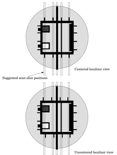
Set up the scan slices so they run through the center of the opposed ramp protrusions for each plane that you would like to view. All the test planes within the cube are spaced in 2.5cm increments. Once you have located the center of any test plane, you can locate the other test planes by indexing 2.5cm.
